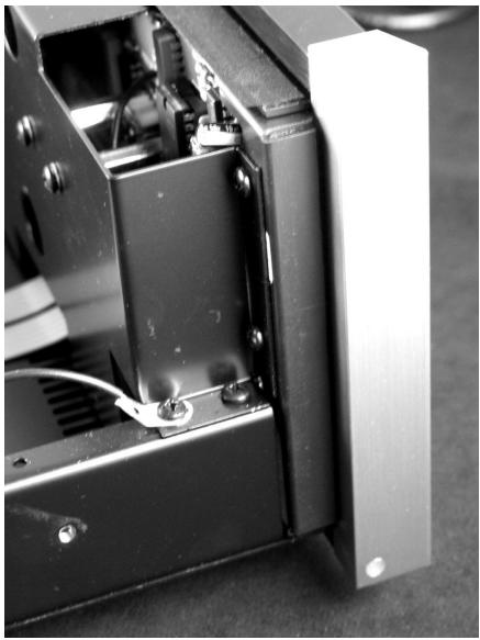
5. There are eight lamps that illuminate the front panel and these must be removed at this time. To do so you will need a  $\frac{1}{4}$ " straight bladed screwdriver. Turn them about  $\frac{1}{4}$  turn counterclockwise and lift them out. There are a few that are buried under the ribbon cables. You will need to gently move the ribbon cable to the side to remove the lamps. The lamps may be lifted out with a pair of tweezers.
