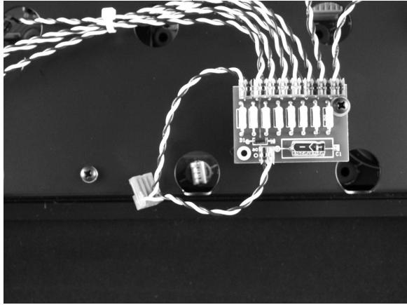
10. Install the seven lamps that are attached to the power supply, in the grommets that were installed in step 6. Slide the lamps into the grommets until the blue lamp socket contacts the grommet. Firmly press down on the blue connector while you wiggle the connector in a circular motion. You may have to moisten them a bit to get them to slide into the grommets.
