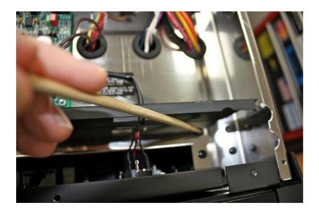
Locate this screw on each lower side of the front panel and remove. The panel should now be free from the chassis.
