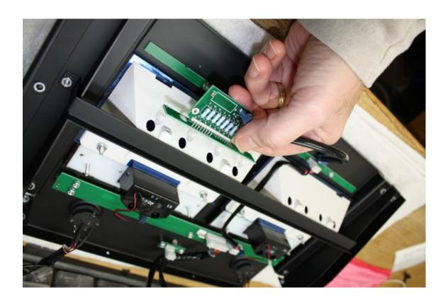
Now install the left meter LED board and wire as shown.
