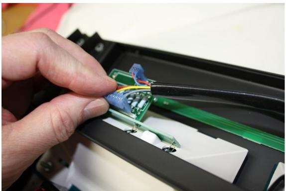
Below the meters you will see the PC board for nomenclature illumination. Using the 1/4 inch nut driver, remove this board and discard. Replace it with the new board that has the same appearance and snug the nuts into place. Do not over tighten.
