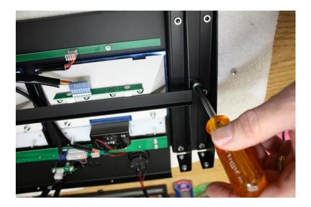
Remove the two 5/16 nuts per meter housing. Remove both white plastic meter housings and set aside. Remove the original blue film filters and replace with ours supplied in the kit. Reassemble this section.
