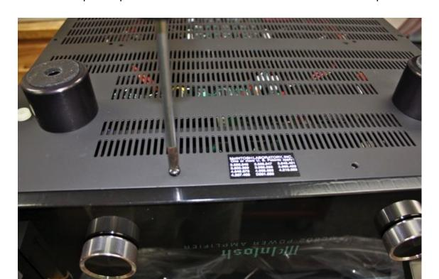
Once the bottom cover is removed you will find the white connectors that run from the PC board to the front panel. There are 4 as I have pointed out in the photos below. Locate these and disconnect. Once they are disconnected from the board, feed them back through the metal framing for ease of panel detachment. See photos below.
