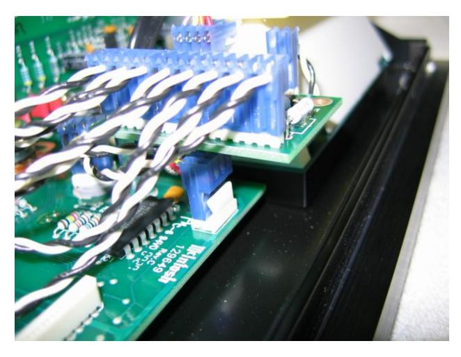
Now remove stock lighting on front panel board, DS15 through DS23 (gray plastic bulb's, eight total) by inserting a straight screwdriver and counter turn 1/4 turn. Replace bulbs with rubber grommet. LED's will insert here as pictured.
