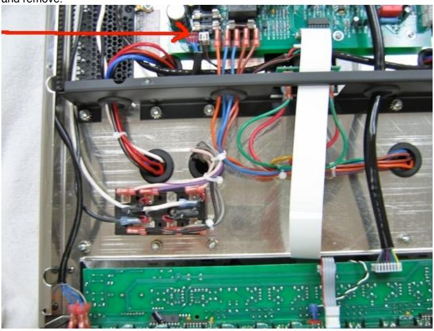
Disconnect the black cable that runs from the front panel to the rear of the unit. Disconnect the white ribbon cable from amp.
