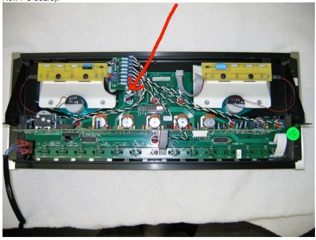
Lamp DS16 accepts the main power from board as pictured in this position. Connect LED Octopus cable as pictured noting polarity.
