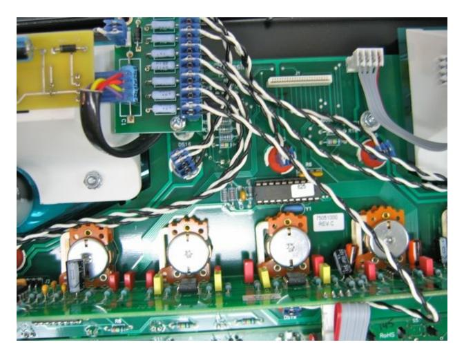
Remove both meter housings (white) by removing chrome nuts. Discard stock filters (blue film sheets) with new filters supplied in kit (green film filter sheets).
