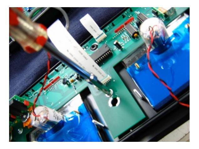
Install the power source for our kit in the bulb location near DS17. The black markings should be towards the top of the panel. This also has a single LED attached.
