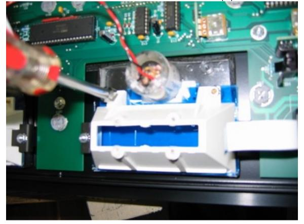
Lift white meter shroud off each meter and remove blue film papers from each
