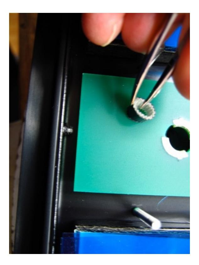
Install the orange rubber grommets where the bulbs once were. Omit DS17, this is where the main LED goes.
