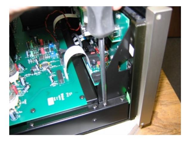
Turn unit over and remove the 3 screws on the bottom panel near the front.
