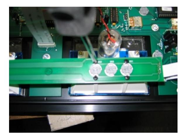
Remove the 1/4" silver nuts attaching the white shroud to the meter.
