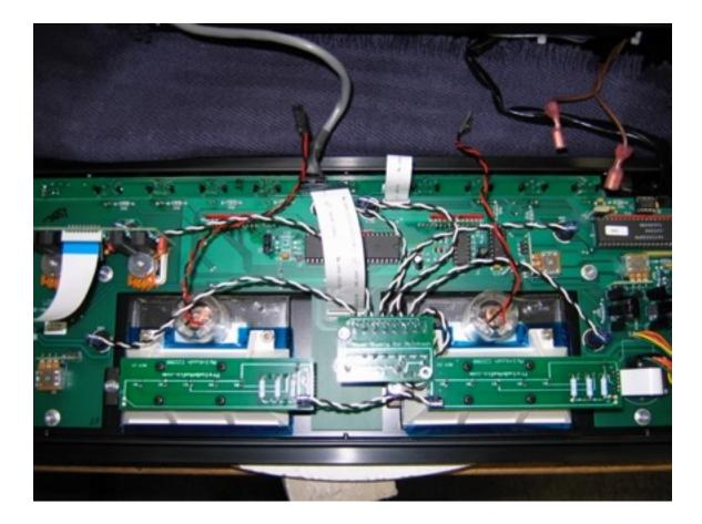
Carefully insert the LED's in there corresponding positions making sure the LED is seated while keeping the rubber grommets in position. Sometimes it is helpful to have a light lubricant on the LED's for easy installation. Also a fingernail holding the grommet doesn't hurt.
