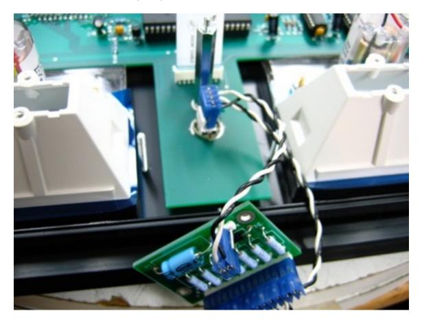
Attach both meter LED assemblies as shown making sure the white ribbon cable is re-attached.
