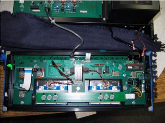
Remove the eight small philips screws that attach the meter illumination PC board to the meters, then disconnect the white ribbon cable.
